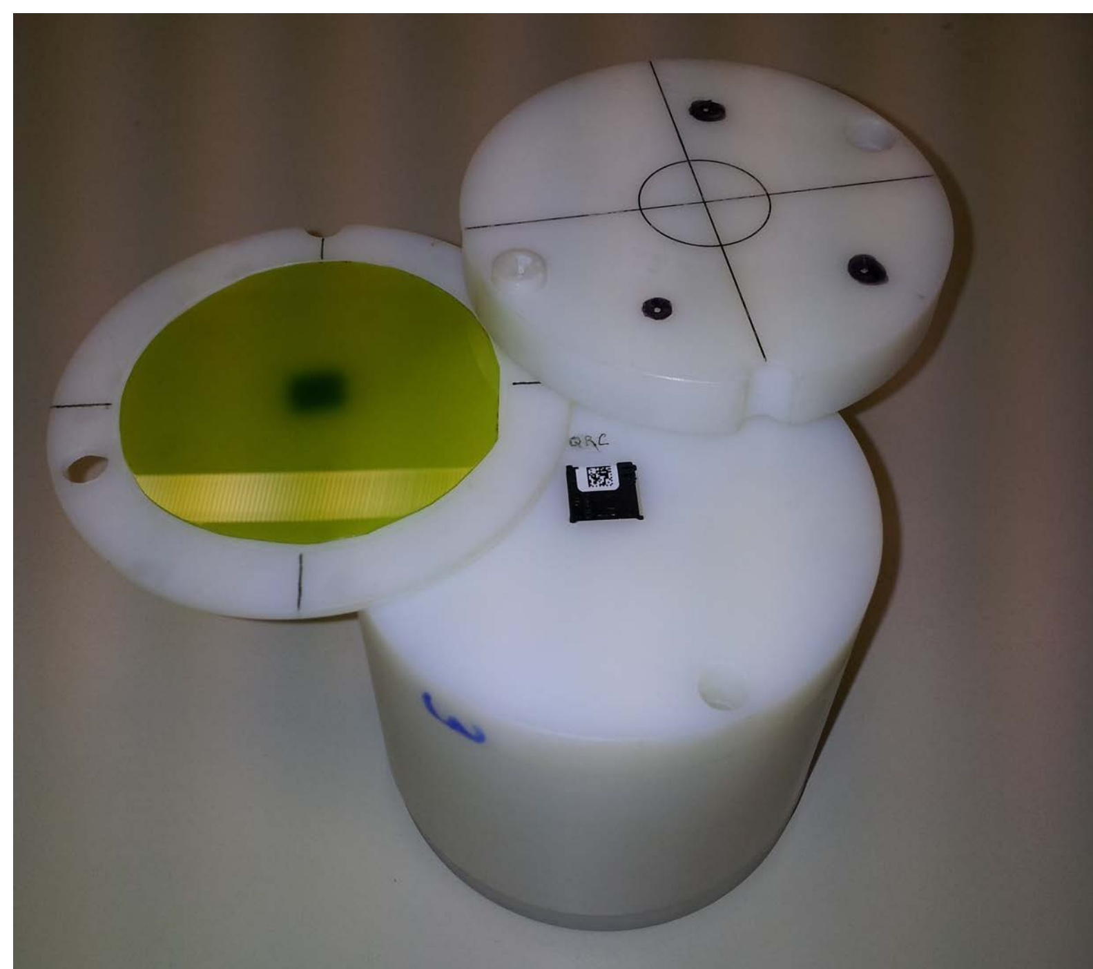
Figure 2: The phantom prototype cone insert with film and OSLDs housing
